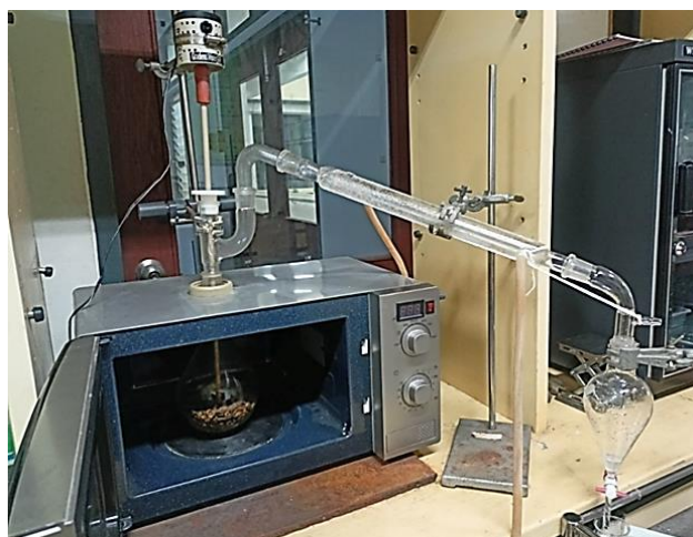
Fig. 1: Solvent-free microwave extraction (SFME) apparatus with an overhead stirrer.
