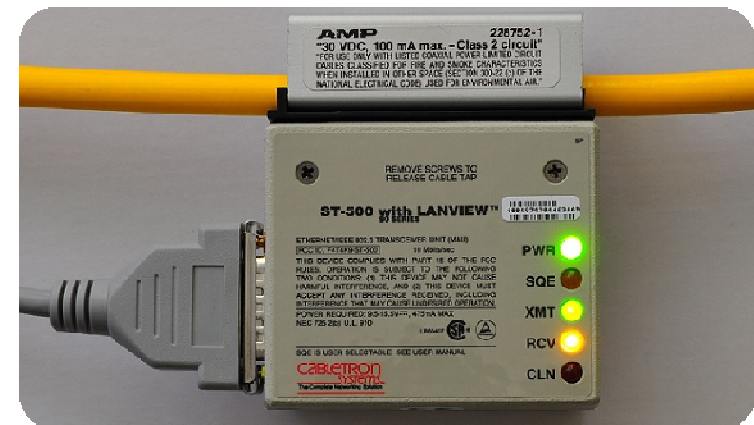
Figure 3-4 Thicknet cable transceiver with detail of a vampire tap piercing the core
