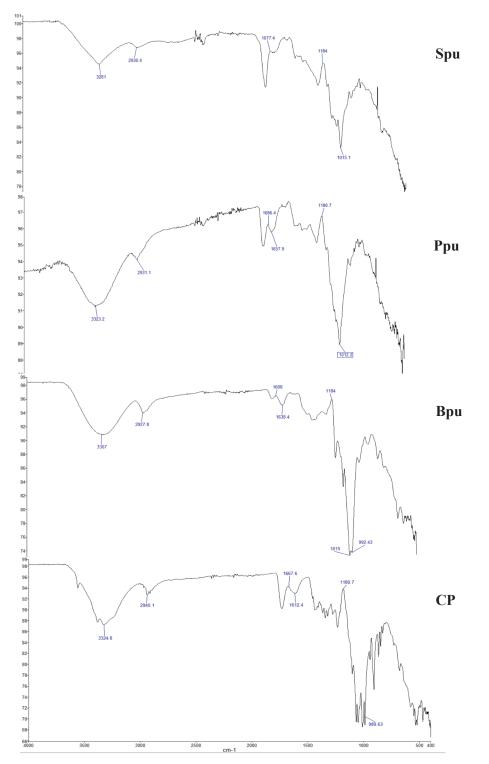
Figure 1. FT-IR spectra of extracted pectin from pulp of indigenous fruits compared to commercial pectin
